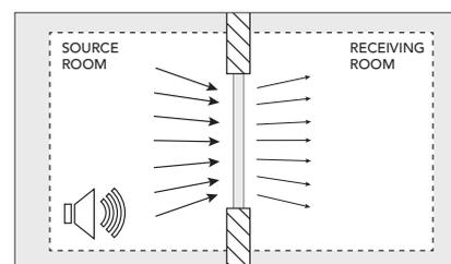
*Typical arrangement for airborne sound transmission testing*
