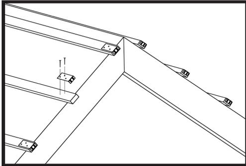
2. Batten end clips (code HD IDV/BC) should be used at the batten ends to provide long term secure fixing. One clip should be nailed twice to the top of each batten with the short flange in contact with the batten end.
