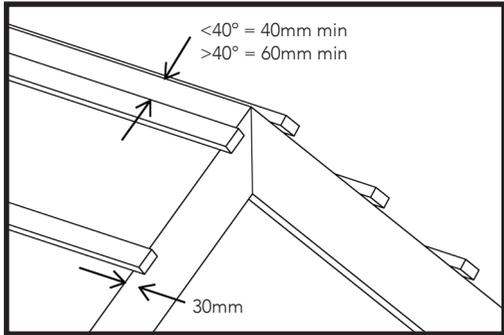
1. The tiling battens should be set out and fixed as required leaving a 30mm overhang beyond the face of the masonry or barge board. The distance between the apex of the rafters and the top batten varies depending on the roof pitch (see diagram above). The roofing underlay should be trimmed along the verge to extend 5mm beyond the ends of the battens.
