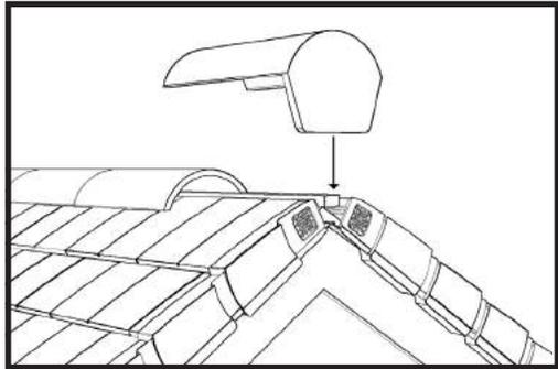
8. Alternatively, a block end ridge tile may be used to complete the installation, fitted in accordance with the tile manufacturer's recommendations. For roof pitches above 50° a block end ridge tile should be used.
