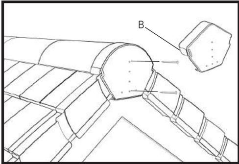
7. The half-round ridge end cap (code HD IPTDV/HR) or universal angle ridge end cap (code HD IPTDV/AR) should be fitted to the ridge tile, interlocking with the verge units and then fixed into the barge board or masonry through the blind holes using the two 65mm screws provided. Extra fixings may be required to secure ridge cap when used on steep roof pitches. For shallow angle ridge tiles, the angle ridge end cap incorporates snap-out tabs (B) for an improved fit.
