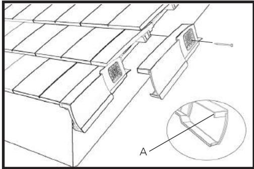
5. Subsequent units are fitted in the same way, clipping each verge unit over the previously fixed unit up to the ridge ensuring that each verge unit is pushed up-slope to fit snugly onto the tile. A small gap of a few millimetres should be maintained between the underside of the dry verge units and the masonry or barge board. When fitting the verge to Forticrete Gemini or Minislate tiles, the tab may be trimmed at A to improve the appearance if required.
