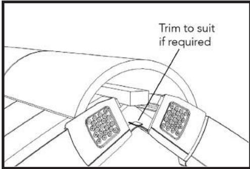
6. When installing at steeper roof pitches, the underside verge closure tabs may require trimming to avoid interference.
