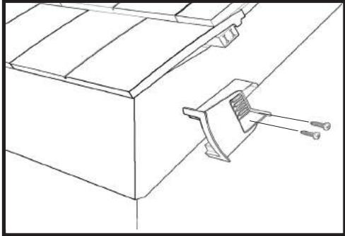
3. The verge starter unit (code HD IPTDV/ST) should be fixed securely at the eaves through the slots using the 2 x 25mm flange head screws provided into the barge board or masonry. The starter unit is most easily marked for position by fitting to a verge unit and placing the verge unit onto the eaves tile.
