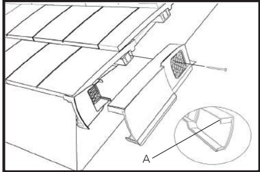
4. Next, clip the first verge unit on to the starter unit; this will require the tab on the first verge unit to be trimmed off at cut line A. Once securely clipped, the verge unit can then be nailed through one of the holes provided into the batten end. Where the batten end clip is used, the nail should penetrate one of the slots provided.
