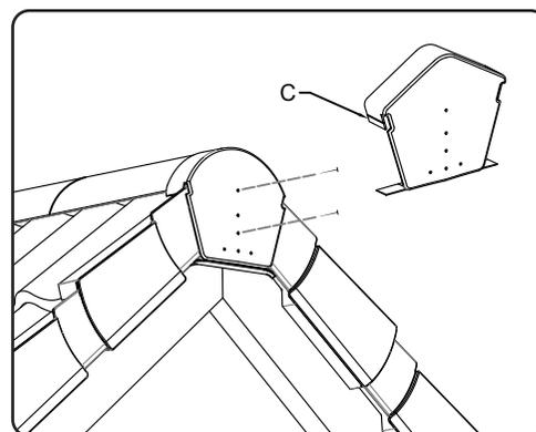
7. The half-round ridge end cap (code HD IDV/HR) or universal angle ridge end cap (code HD IDV/AR) should be fitted to the ridge tile, interlocking with the verge units and then fixed into the barge board or masonry through the blind holes using the two 65mm screws provided. For shallow angle ridge tiles, the angle ridge end cap incorporates snap-out tabs (C) for an improved fit.
