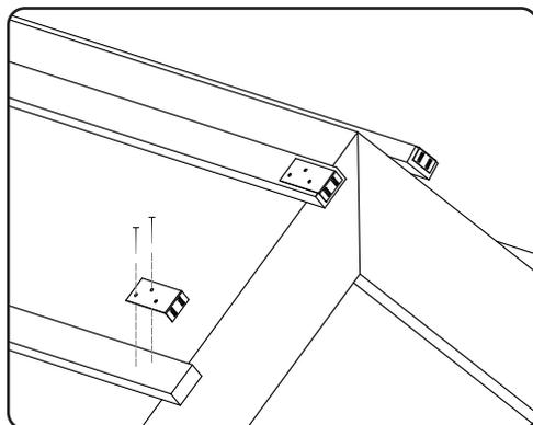
2. It is recommended that batten end clips (code HD IDV/BC) be used at the batten ends to provide long term secure fixing. One clip should be nailed twice to the top of each batten with the short flange in contact with the batten end.
