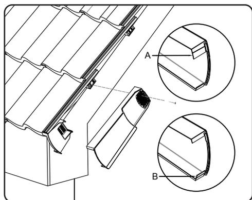
5. Next, clip the first verge unit onto the starter unit; this will require the flange tab A (code HD IDV) or B (code HD TIDV) on the first verge unit to be snapped off at the break line. Once firmly clipped to the starter unit, the verge unit can then be nailed through one of the holes provided in the batten end or continuous batten. Where the batten end clip is used, the nail should penetrate one of the slots provided.
