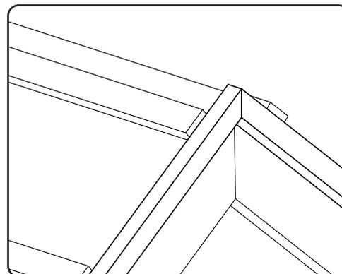
3. For refurbishment installations where the batten end clip cannot be fixed without removing the tiles, or where the batten ends are not exposed or have decayed, fix a 35mm or 38mm thick continuous batten along the length of the verge to provide an alternative fixing for the verge units. Fixing into or with mortar is not recommended.
