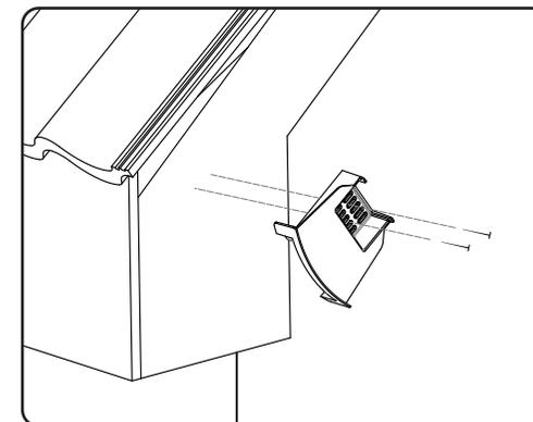
4. The verge starter unit (code HD IDV/ST) should be fixed securely at the eaves through the slots using the 2 x 25mm flange head screws provided into the barge board or masonry. The starter unit is most easily marked for position by fitting to a verge unit and placing the verge unit onto the eaves tile.
