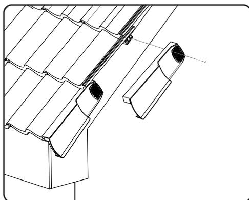
6. Subsequent units are fitted in the same way, clipping each verge unit over the previously fixed unit up to the ridge ensuring that the verge unit is pushed up-slope to fit snugly onto the tile. A small gap of a few millimetres should be maintained between the underside of the dry verge units and the masonry or barge board.
