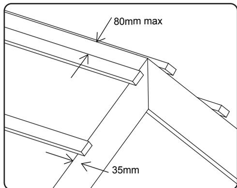
1. The tiling batten should be set out and fixed as required leaving a 35mm overhang beyond the face of the masonry or barge board. The distance between the apex of the rafters and the top batten should not exceed 80mm. The roofing underlay should be trimmed to extend 5mm beyond the ends of the battens.
